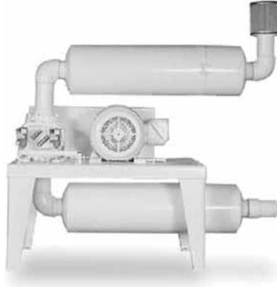
**Pressure Blowers - Vacuum Blowers for Pneumatic Conveying Systems - Flour and Sugar Systems**
